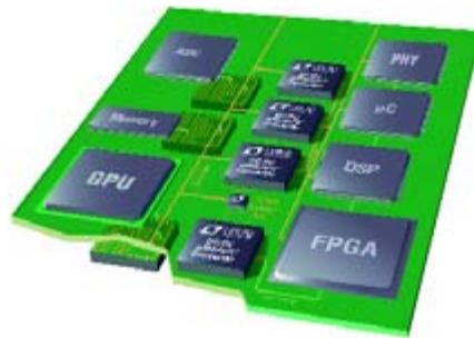
Figure 1 - A \mu Module DC/DC converter is a complete power supply solution small and light weight to fit on top and/or bottom of a PCB leaving room for digital ICs.
