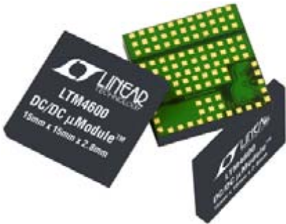
Figure 6 - Thermally enhanced packaging delivers very high power density switchmode DC/DC conversion in 15mm x 15 mm x 2.8mm surfacemount LGA package
