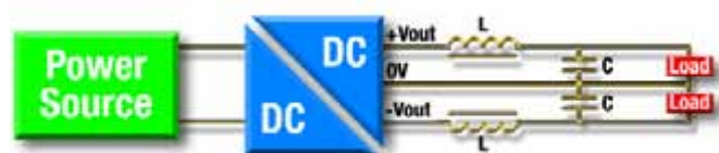
Figure 2: Output filter design for dual-output NMJ-series DC-DC converter.
